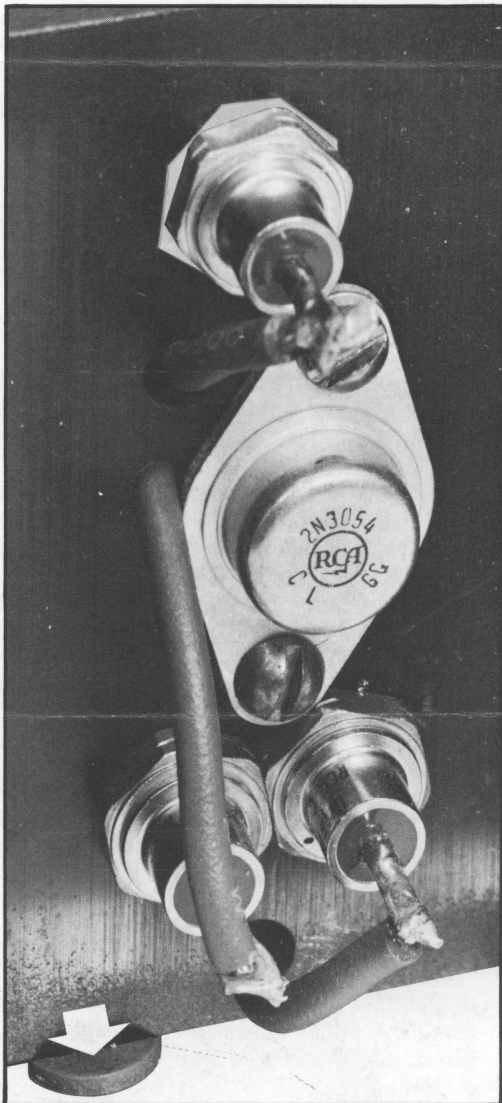
Figure 4: Closeup of left side of heat sink shows how it is insulated from the chassis by fiber shoulder washer (arrow). Note how hexagonal mica insulator is placed under diode, D_1 , shown at top. The same arrangement should be used in mounting diode, D_4 , on the right side of the heat sink.
